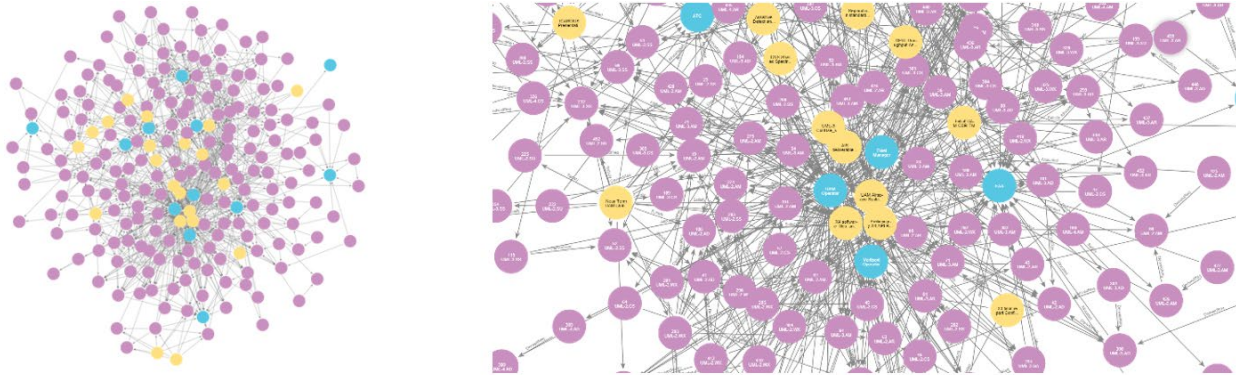
Fig. 1 Partial UAM Knowledge Graph Structure relevant to this study where purple nodes are requirements, blue nodes are system actors, and yellow nodes are project's deliverables (the left figure for the bird-eye view and the right for the zoom-in view)
