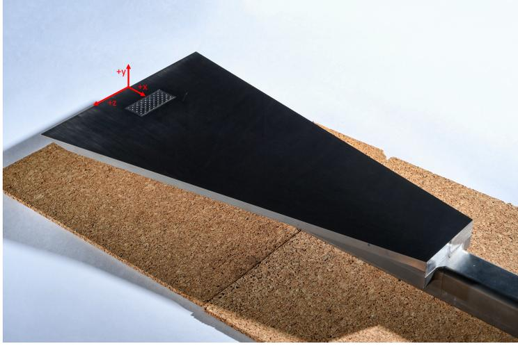
**Fig. 4 Flat plate model with coordinate system in red. [Credit: NASA]**
