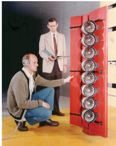
Figure 2: Blown Flap Model in NASA Lewis 9- by 15-Ft Low Speed Wind Tunnel. Image: NASA 1970-C-01199
