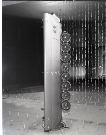
Figure 3: Fan-on-Flap Model in NASA Lewis 9- by 15-Ft Low Speed Wind Tunnel. Image: NASA C-1970-02412
