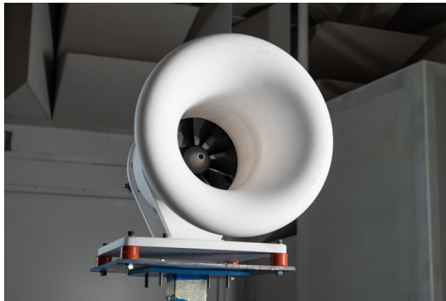
Figure 10: Photograph of the QUEEN V1 test set-up in the NASA GRC Acoustical Testing Laboratory, forward looking aft.
