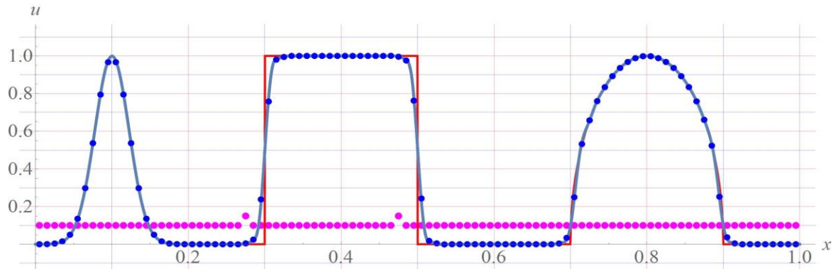
(c) DG3 solution with limiting and \sigma = 0.125 after 800 time steps (distance travelled: 1 period)
