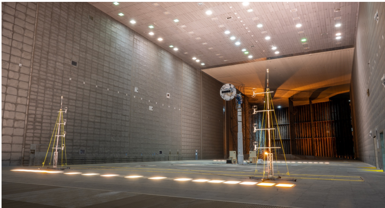
Figure 10 Test section with two towers upstream of model, each equipped with 4 RM Young 81000 ultrasonic anemometers
