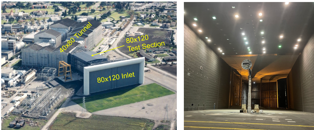
Figure 2 NFAC facility (left) and 80x120-foot test section with Dragonfly test article (right)
