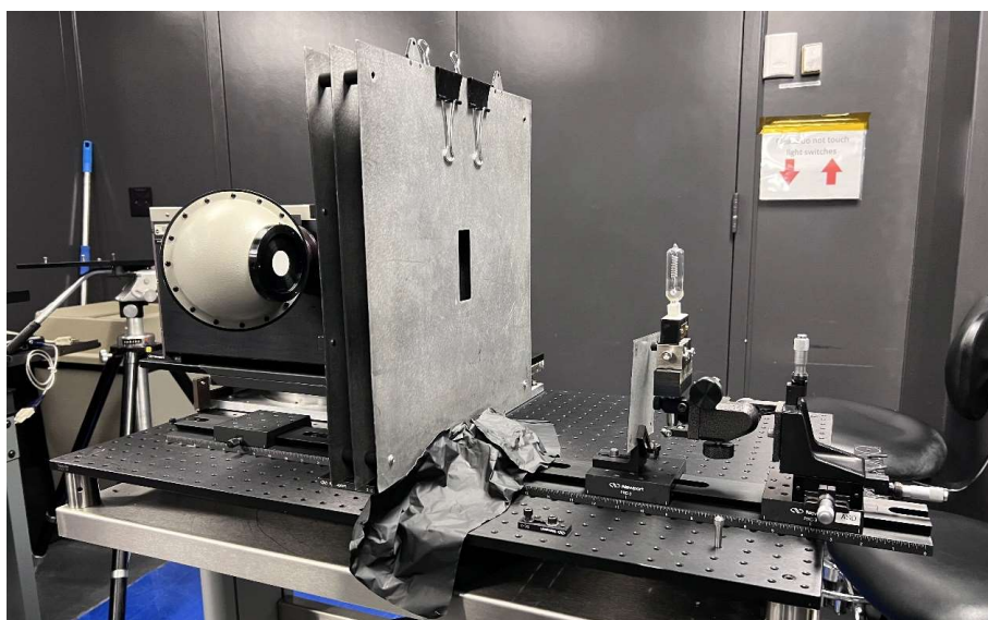
OL 750 calibration setup with standard lamp NIST supplied spectral irradiance at 50 cm
