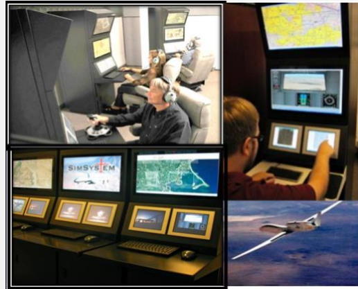
Figure 4: Remotely Piloted Aircraft System (ground control station) Synthetic Task Environment used for research
