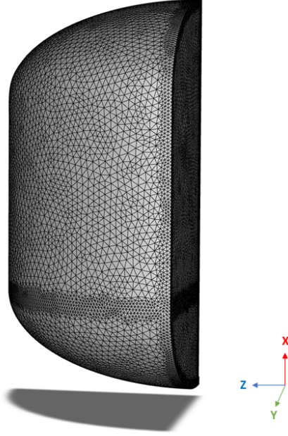
Fig. 2 Computational mesh for the 25% fill ratio spray-bar mixing case (256,729 cells).
