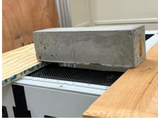
Figure 7. Photograph of sample A being oriented on the backscatter x-ray system.
