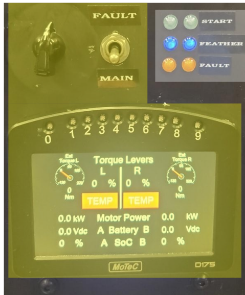
Fig. 9 The X-57 pilot-in-the-loop simulator multifunction display (yellow shaded box) and propeller indicator lights (white box).
