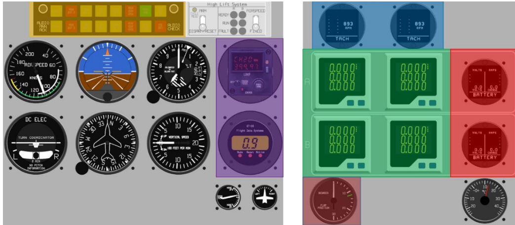
Fig. 8 The X-57 piloted simulator heads down display (HDD): (left) panel includes stock P2006T instruments (no shading); annunciator panel (orange shading); high-lift system control switches (white shading); radio (top purple shading); and accelerometer (G-meter) (bottom purple shading); and (right) panel includes tachometers (blue shading); avionics power meters (red shading); flap indicator (brown shading); and battery power meters (green shading).
