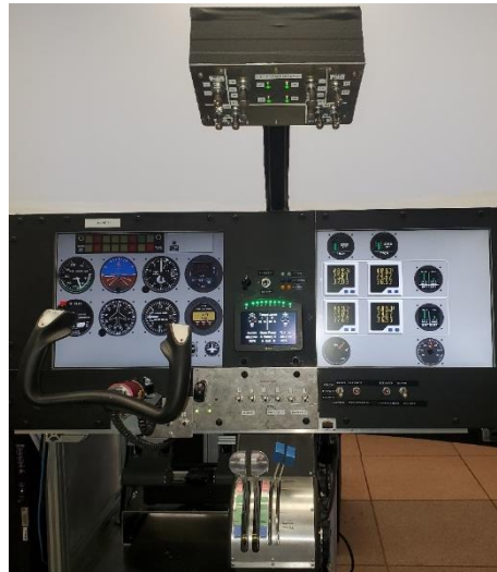
Fig. 7 The X-57 pilot-in-the-loop simulator cockpit dashboard, control surface inceptors, motor power control inceptors, and overhead switch panel.
