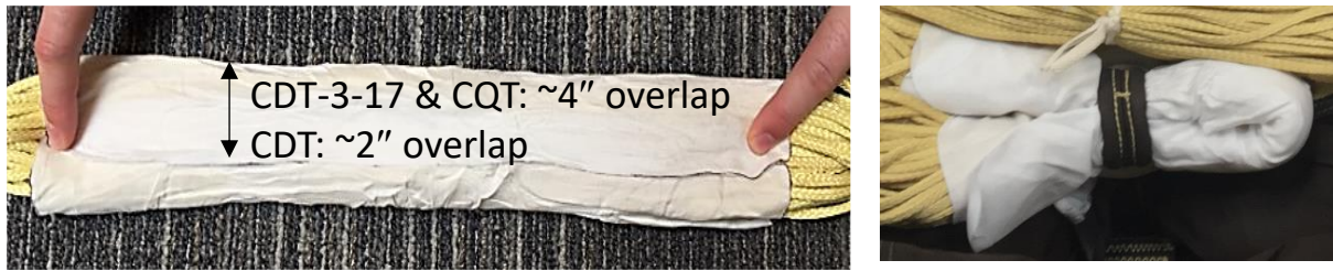
Figure 5. CPAS bight sleeve wrapped around suspension lines with overlap (left) and stowed (right).
