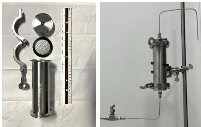
Figure 2. The parts and the assembled stainless steel prototype cell.
