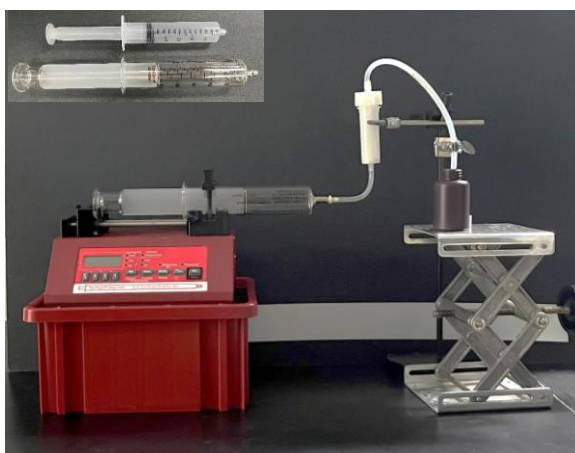
Figure 4. The flow-through test setup at 0.4 mL/min with a glass syringe. The insert image shows both the plastic syringe and the glass syringe.
