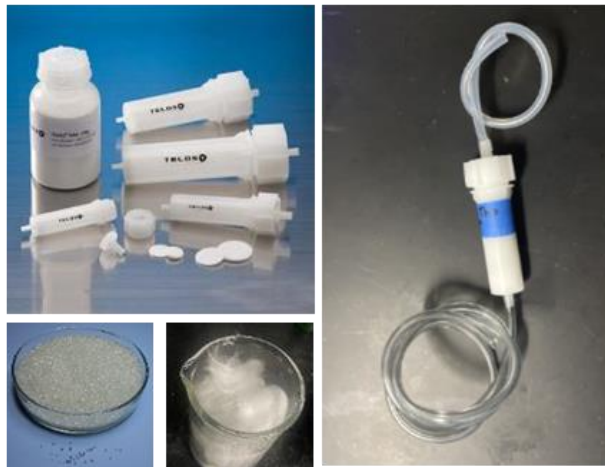
Figure 1. The first-generation plastic-packed bed cell is built with a TELOS cartridge, glass beads, and quartz wool.
