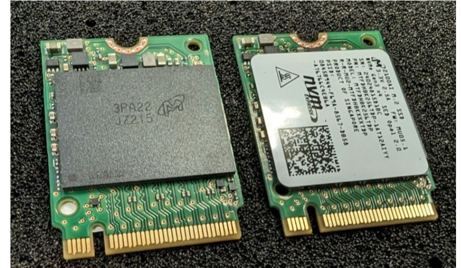
Ex: Micron 2100AT +105° C, Up to 1 TB in BGA Configurable SLC or TLC
