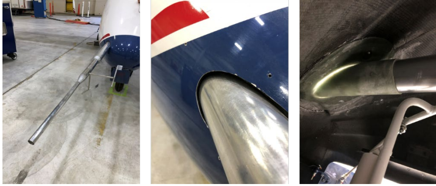
Fig. 3 The air data probe (left to right: overview, closeup view, inside view).
