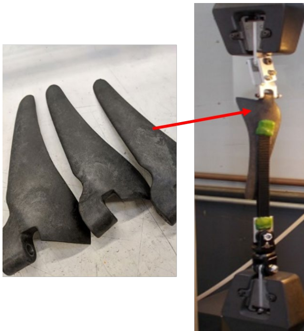
Fig. 16 The X-57 Mod IV high-lift blade proof test.
