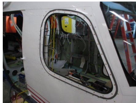
Fig. 7 The secondary egress window.
