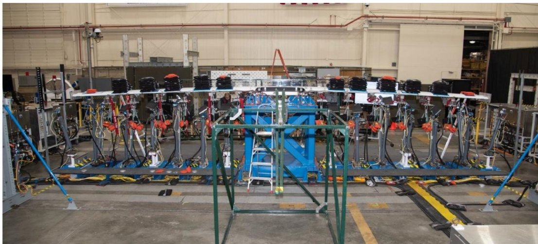
Fig. 12 The X-57 wing shot-bag download testing at maximum load.
