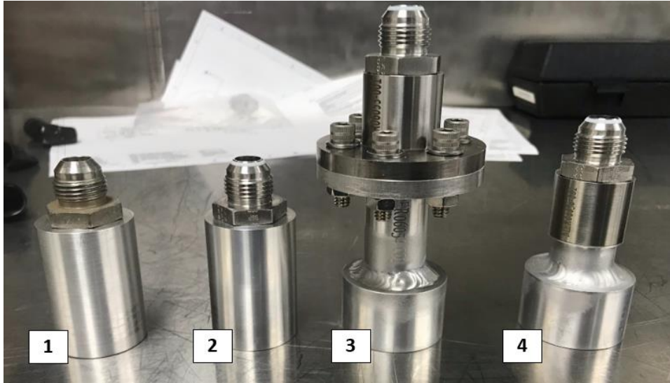
Figure 1. Test fixtures tested for aluminium to stainless-steel joints [1].
