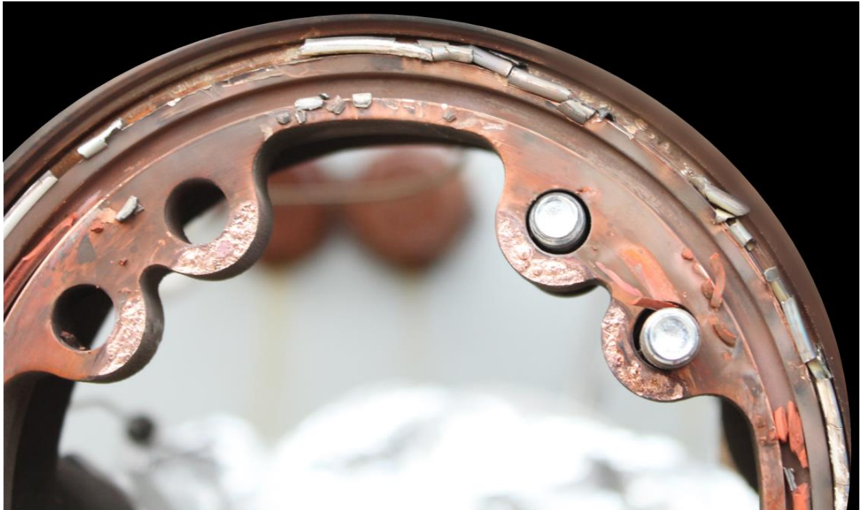
Figure 1. Injector to inner body seal damage post-hot fire test #3.
