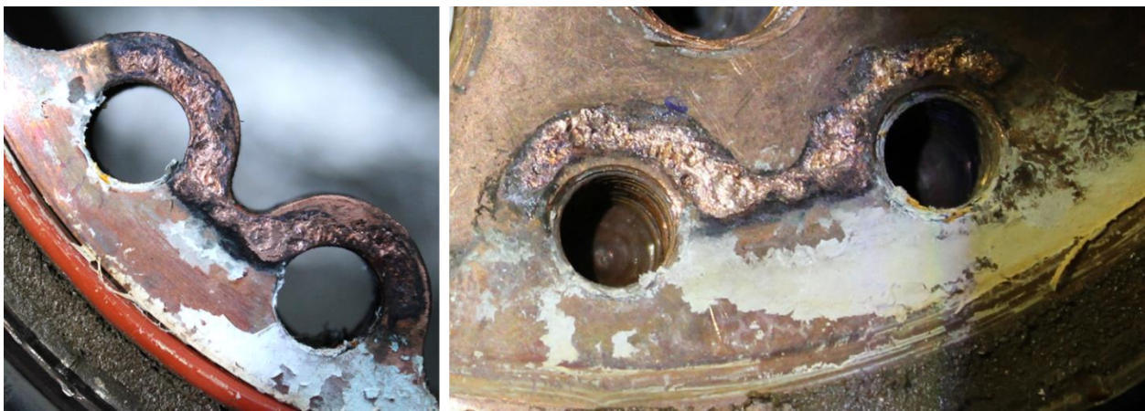
Figure 4. Injector to inner body fusing around the bolt holes post-hot fire test #8.
