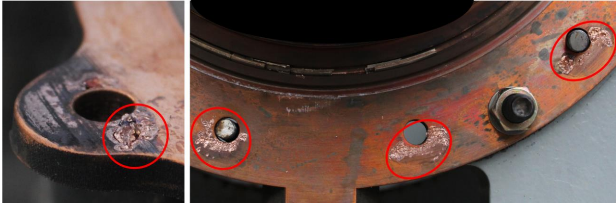
Figure 2. Injector to outer body fusing around bolt holes post-hot fire test #3.
