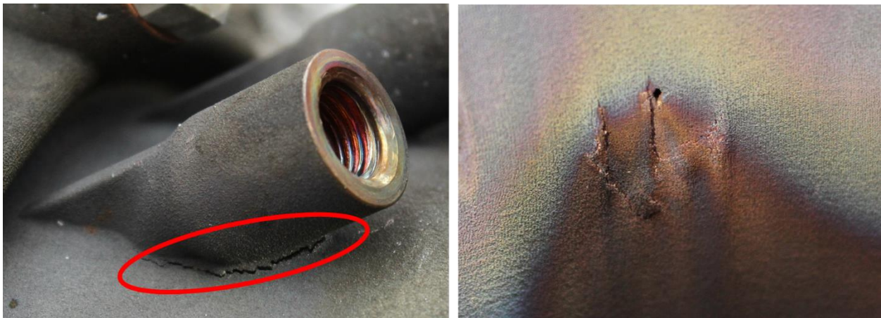
Figure 3. Outer body hot wall static pressure port cracking post-hot fire test #3.
