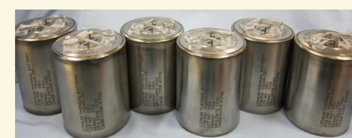
1/3 scale batteries that function at temperatures up to 500 C delivered to GRC for testing by Advanced Thermal Batteries, Inc.
