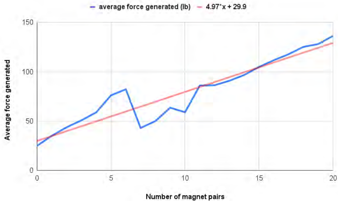
Figure 7: Average force measured per number of magnet pairs on the flywheel
