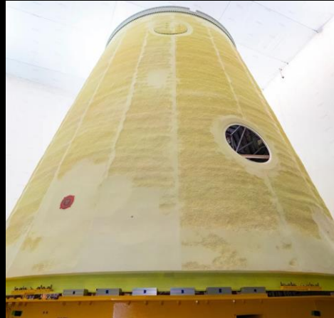
Frangible joint assembly installed onto the Launch Vehicle Stage Adapter
