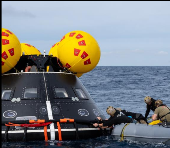
U.S. Navy personnel grab onto a mockup of the Orion spacecraft during a practice procedure of the Underway Recovery Test 11 (URT-11)
