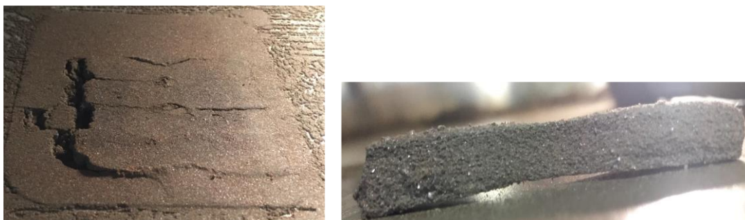
Figure 10. Warping during the build and sample curling post building
