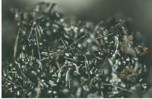
Figure 15. SEM micrograph showed milled carbon fibers at fracture surface
