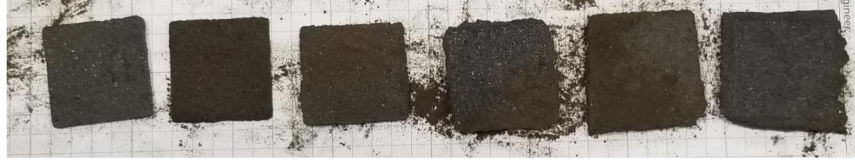
Figure 6. Carbon-fiber-filled RTM370 composite chips by LS
