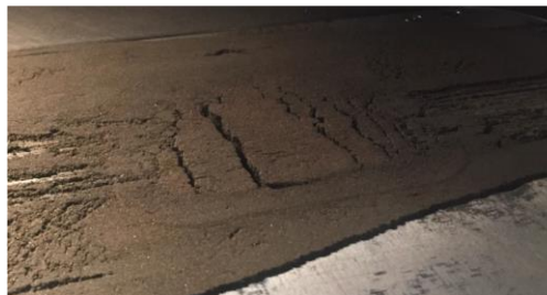
Figure 8. Composite feed bed cracking due to high heat
