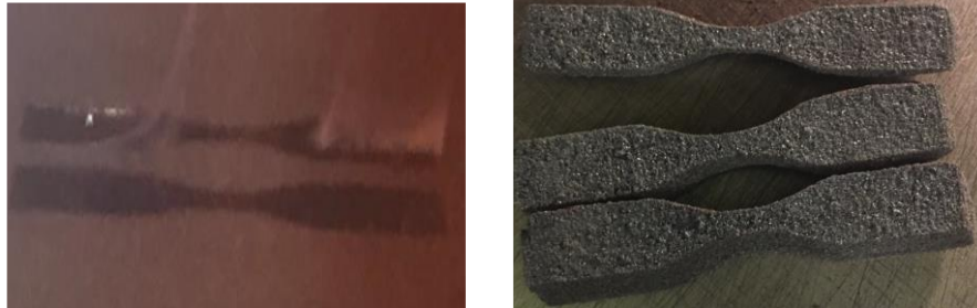
Figure 11. Tensile specimens during LS build process and after post build
