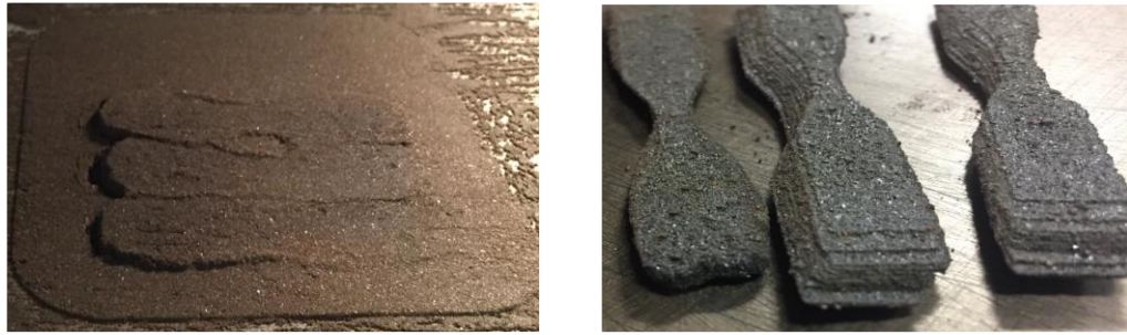
Figure 9. Layers shifting during the build and post building
