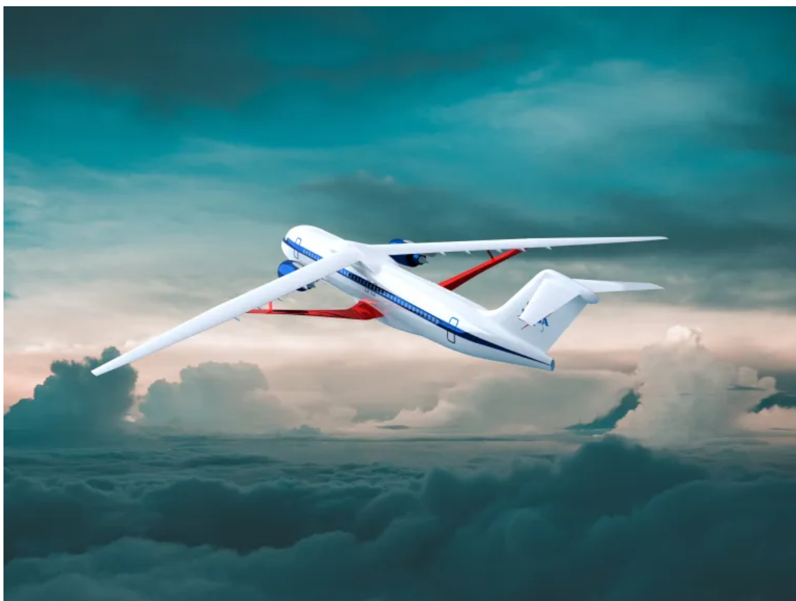
Figure 1 – Artist's rendering of a transonic truss-braced wing concept aircraft.
