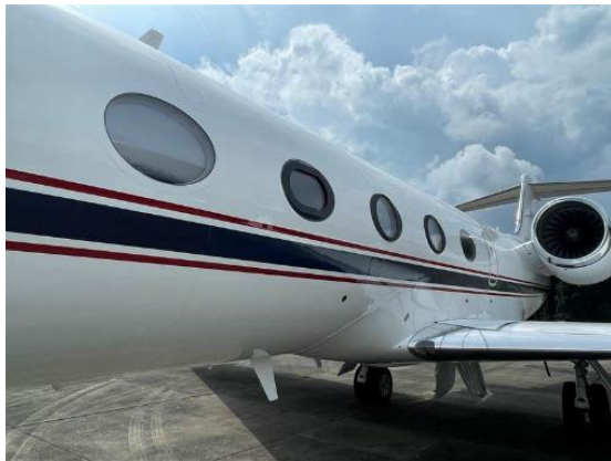
Figure 4. External view of windows on NASA Gulfstream aircraft, left to right: original gulfstream window, previously designed acrylic “racetrack” shaped window, two new fused silica windows, and an original Gulfstream window.
