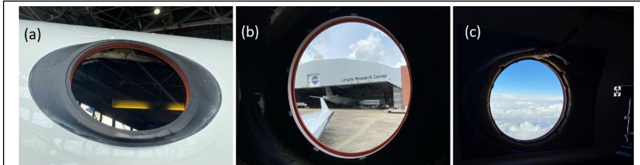
Figure 2. Fused Silica window utilizing a 17-inch diameter (16.4-inch diameter viewable area) with custom frames compatible with Gulfstream window ports and installed on a Gulfstream 4 Aircraft at NASA LaRC: (a) outside view, (b) inside view, and (c) in-flight view during a mission.
