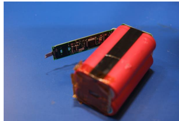
2S2P 18650 COTS Pack Approved for ISS Flight
