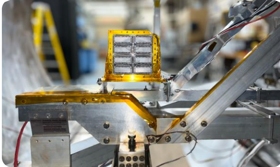
Figure 2. MPT5.0-005 Mounted to Thrust Stand in VF-3 at NASA/GRC (View from Front).
