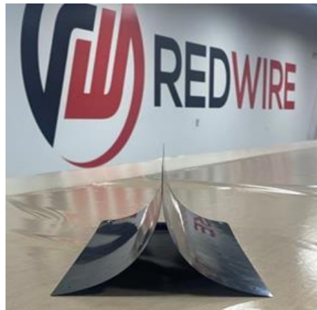
Figure 4. TRAC Boom Cross Section
