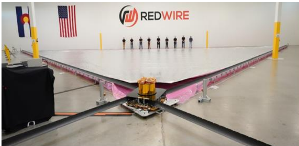
Figure 2. Solar Cruiser TRL 6 Demonstration Unit Following Single Quadrant Deployment Testing
