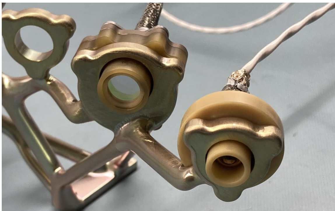
Figure 13. Initial integration of a Photodiode Subassembly ( left ) and LED Subassembly ( right ) to the Sensor Array bracket.
