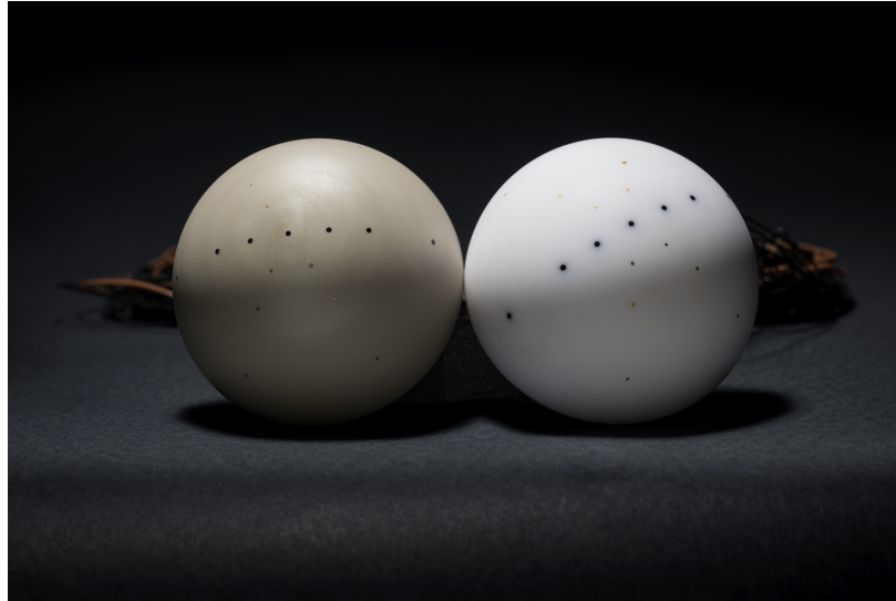
Fig. 1 PEEK (left) and Formlabs Rigid 10K (right) hemisphere models instrumented with Ahmic Aerospace high-speed temperature gauges.
