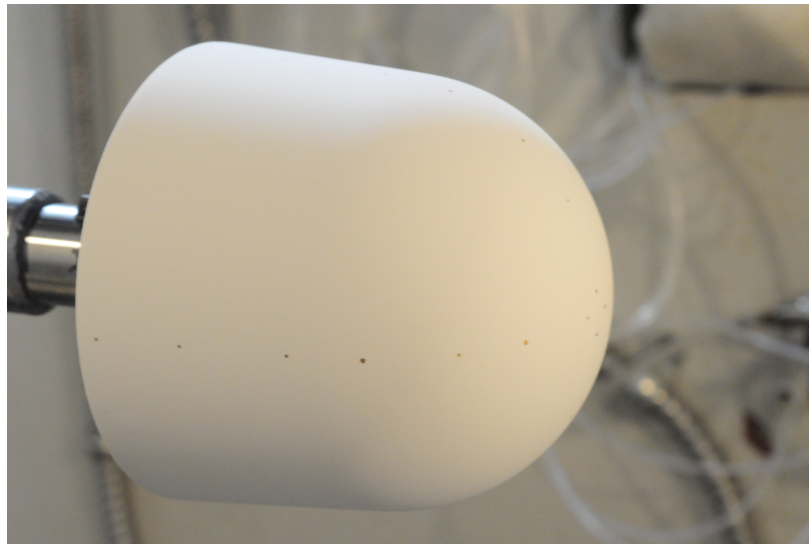
Fig. 2 Slip-cast fused silica ceramic hemisphere-flare model mounted in the injection box beneath the test section.
