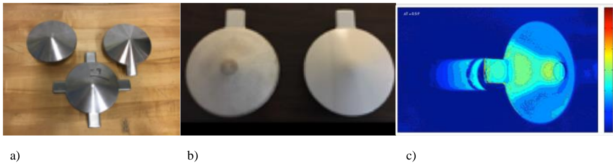
Fig. 23 a) Metallic trim tab models [Photo Source: NASA], b) prototyped models, c) surface IR thermography contour map.
