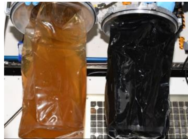
Comparison of UWMS-filled EDV (Russian tank) on left that shows no pretreat and tank previously filled from WHC on right with expected color with pretreated urine.
