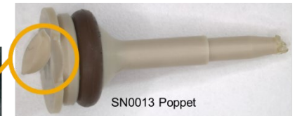
Poppet fractured during nominal handling after removal from SN0013 Valve
