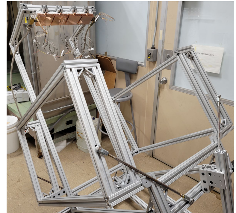
Benchtop solar thermal receiver integrated with solar concentrator (reflectors not shown)
