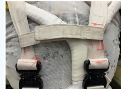
Interior view of the HUT from the top showcasing shoulder strap attachment points (top), shoulder strap sizing (bottom).
