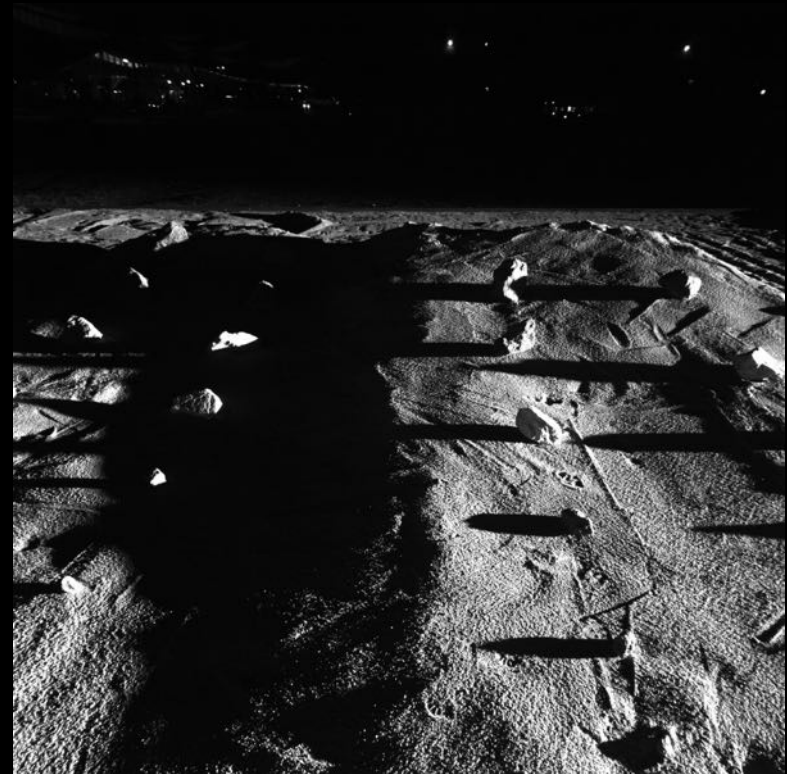
Rock field for hazard map testing with sun simulator on the right
