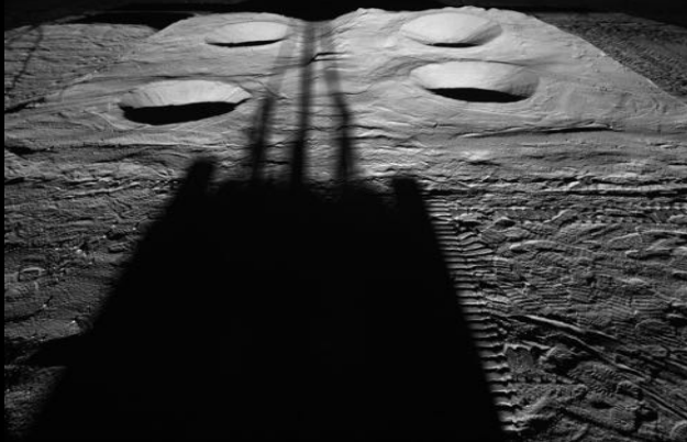
Engineering Unit Rover NavCam view with Sun Simulator from behind
