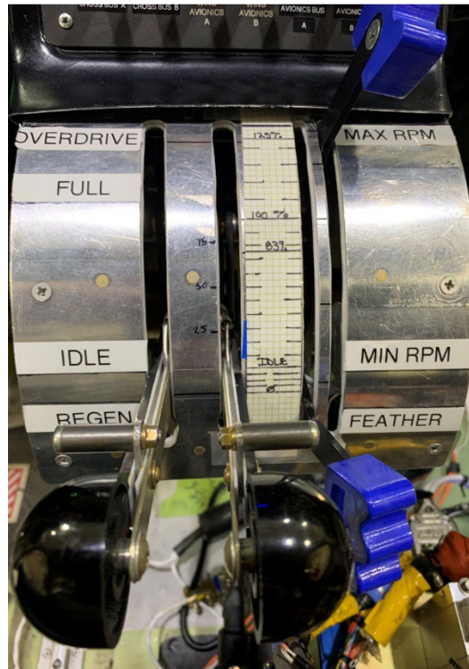
Fig. 2 Torque and propeller pitch levers.
