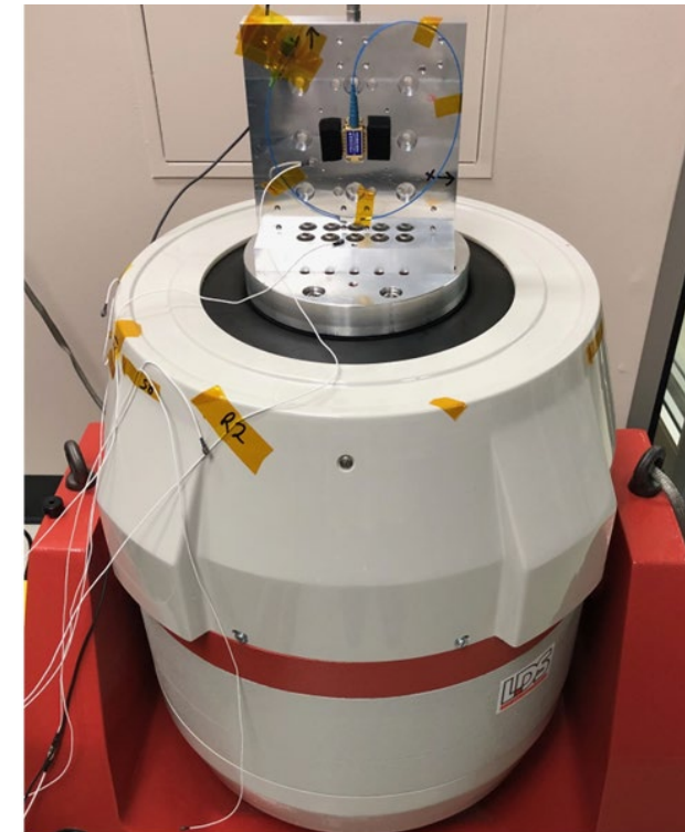
Tunable laser diode in vibration testing
