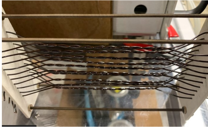
Fig. 5 300TP after seven thermal aging cycles and 207 hours at 300 °C.
