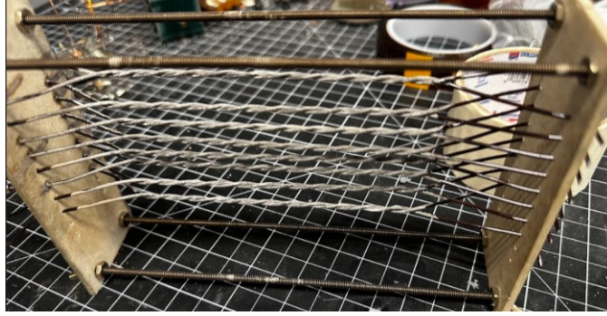
Fig. 10 270CTP after 3 thermal aging cycles.
