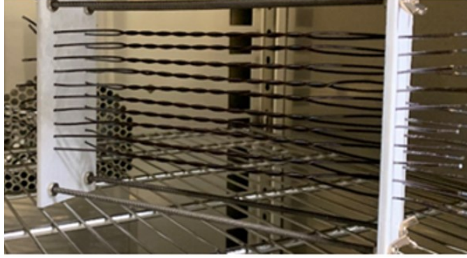
Fig. 4 300TP After 1st Thermal Aging Cycle - 46 Hours at 300 °C.
