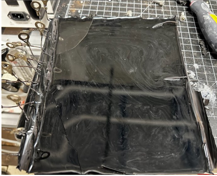
Fig. 20 250TP after 6 aging cycles. Pairs are numbered 1 to 8 from the top of the photo to bottom.
