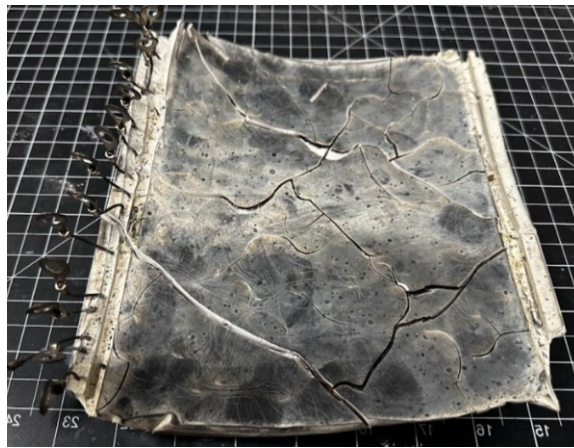
Fig. 15 270PTP after last aging cycle.
