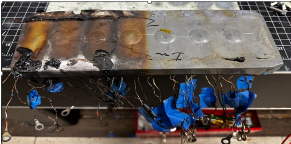
Fig. 31 Motorette number 2 after an accidental \sim 2 day cycle at >250\text{ }^{\circ}\text{C} on coils 1-4. Visual aging of coils 1-4 (left) vs 5-8 (right) provides additional evidence of the lack of thermal coupling between the two halves of the motorette when one half is powered.
