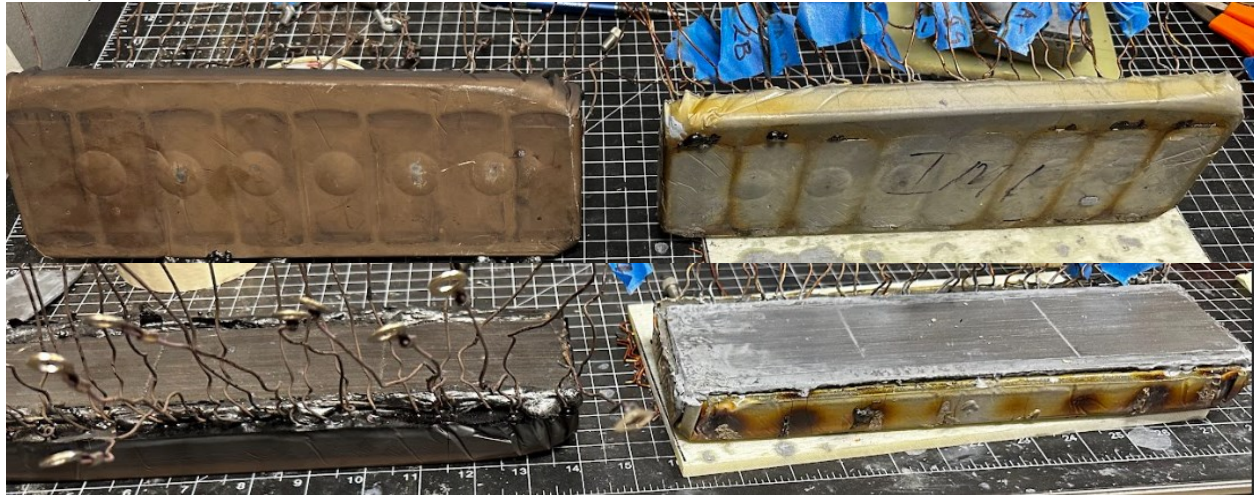
Fig. 40 Motorette 4 (left) and motorette 1 (right) after their aging cycles.
