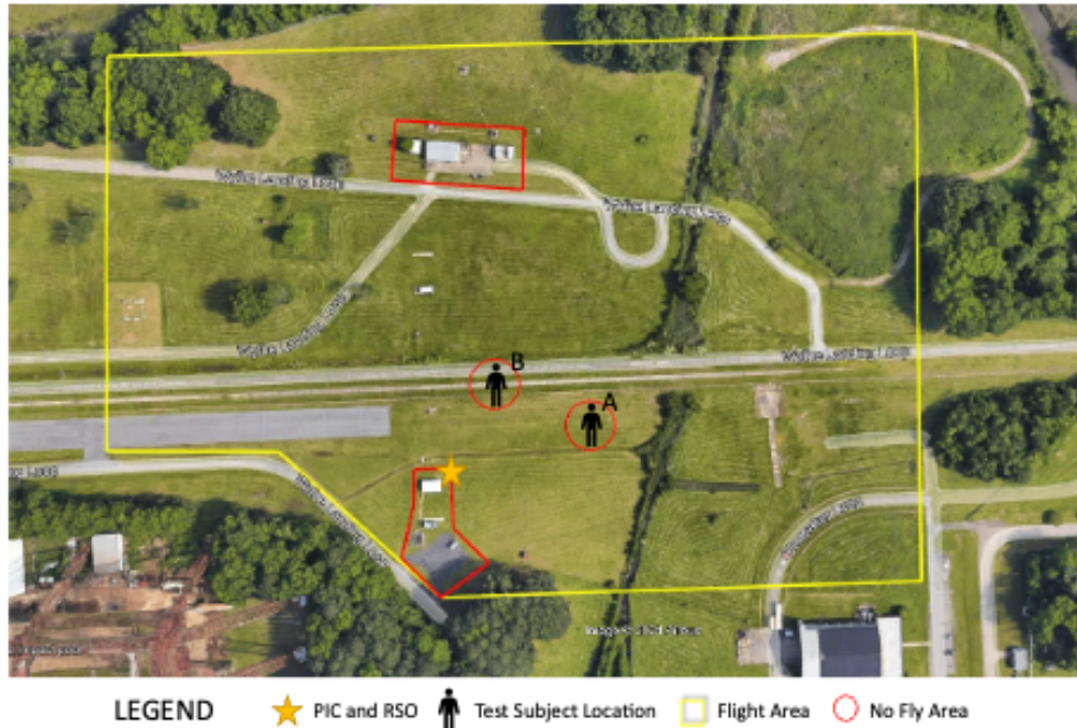
Fig. 2 Approximate locations of ATDs and human participants during data collection flights. Between different configurations, the location was subject to change within 50 feet. Location A identifies an area where the participant was surrounded by a grassy field, and Location B identifies an area where the participant was on a strip of sidewalk with grass on both sides.
