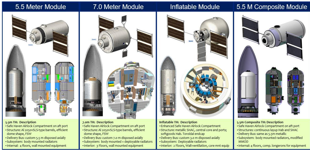
Fig. 1 Four Mars Transit Habitat Configurations Traded
