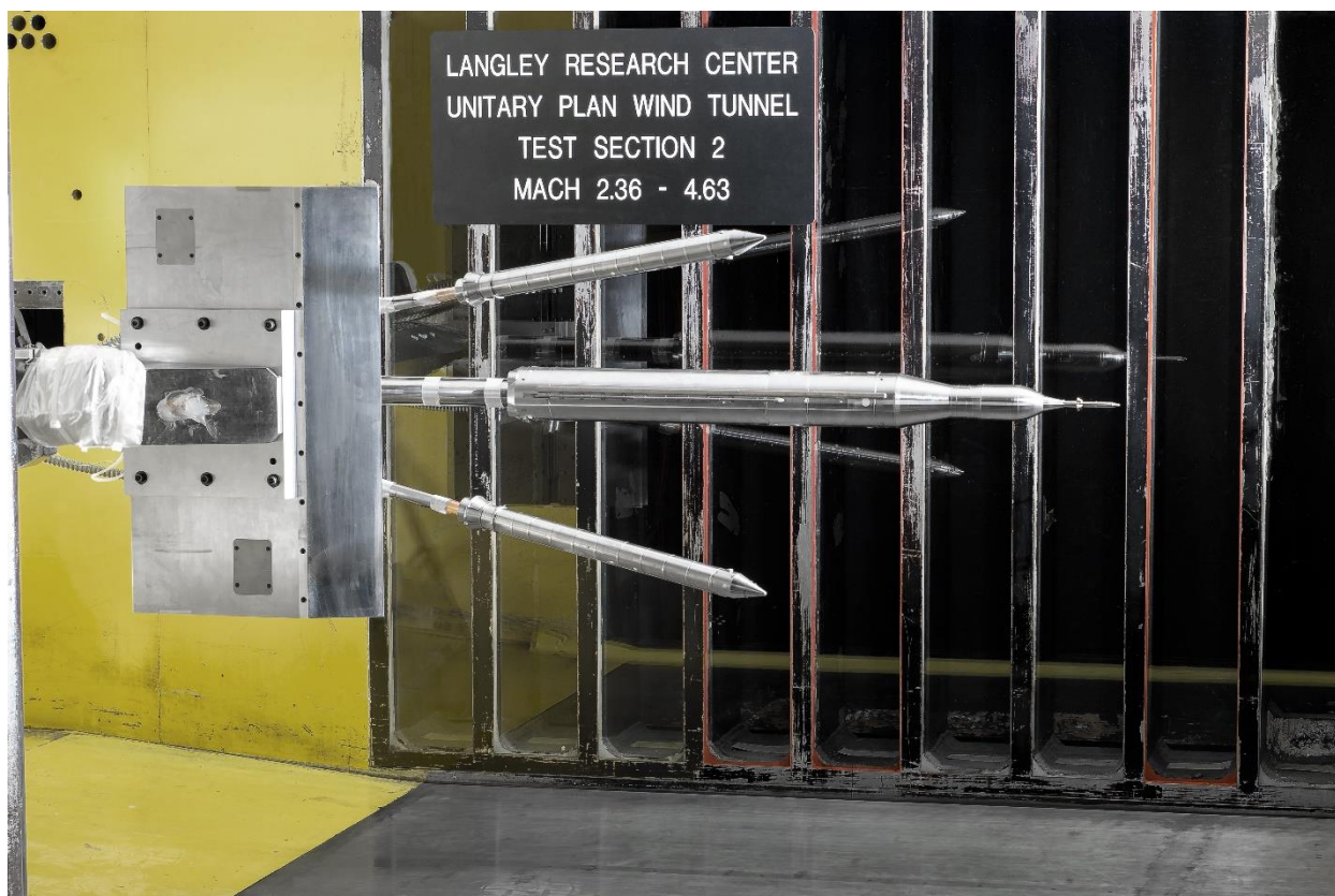
Figure 4. Wind tunnel testing of booster separation. Pressurized air was blown through the solid rocket boosters to simulate the booster separation motors firing.
