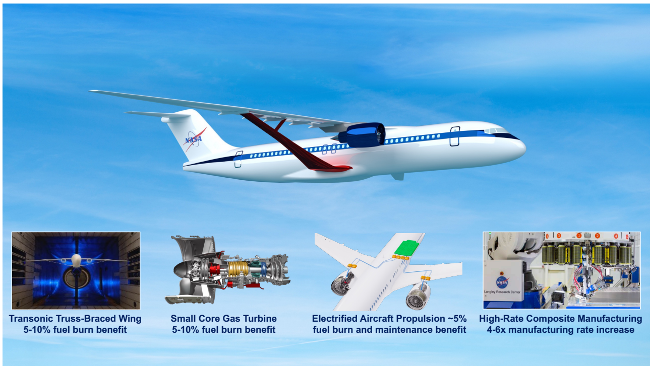
Figure 1 – The NASA AAVP's key demonstrators and technical challenges advancing sustainable aviation technology for the next-generation commercial aircraft (colloquially called the “Fab 4”).
