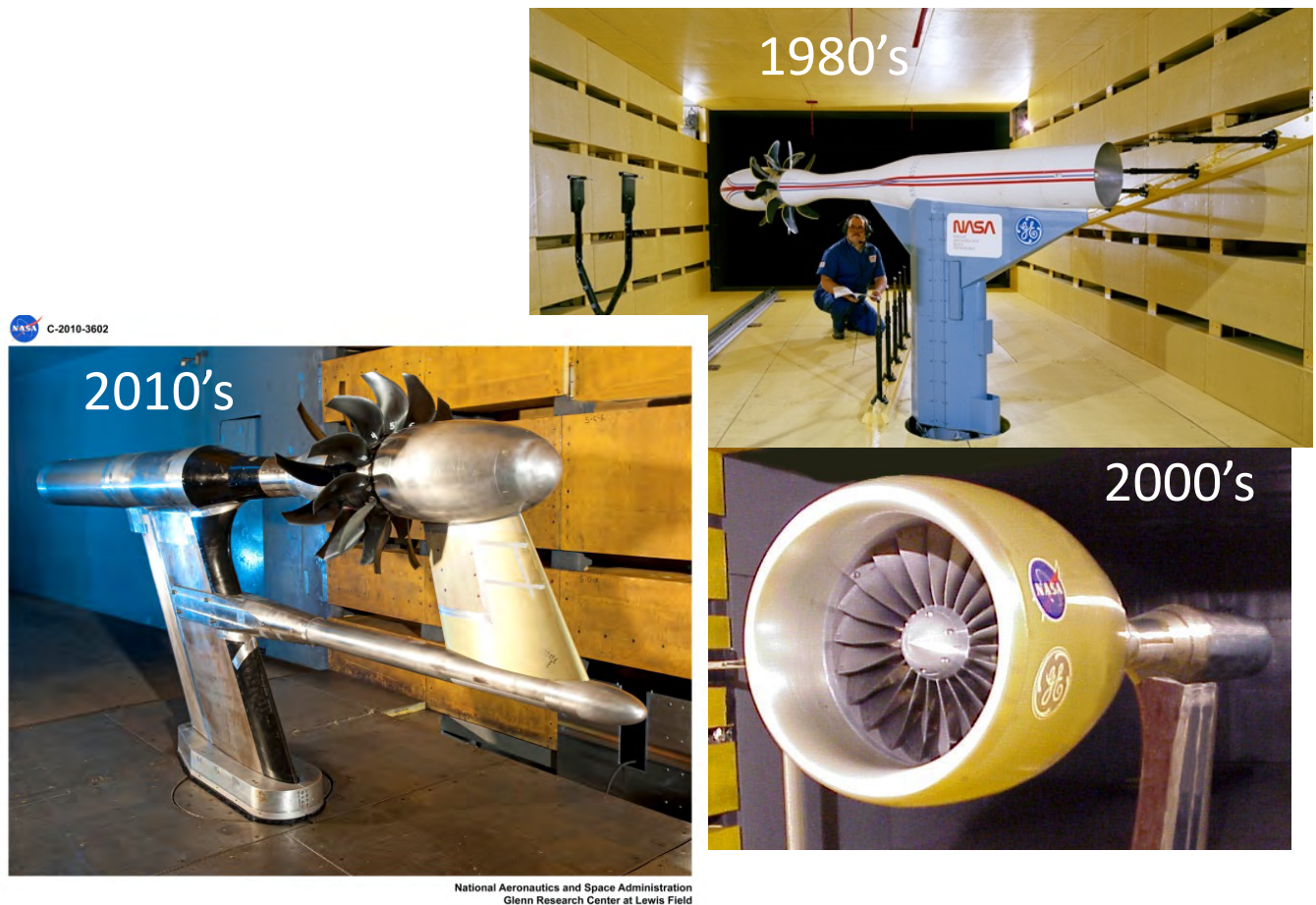
Figure 4 – Pictures from wind tunnel tests in the 9x15 LSWT dating back to the 1980's Un-Ducted Fan (UDF) test.
