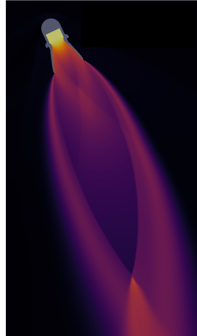
Temperature in a slice through the symmetry plane of a rocket motor.
