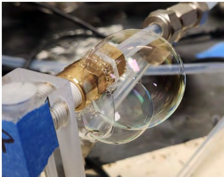
Figure 32: Soap bubble from soap leak test
