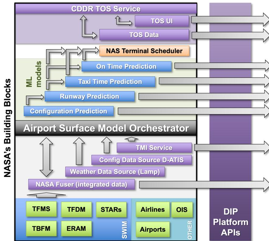
Figure 4 – Predictive engine service-oriented architecture. TFMS: Traffic Flow Management System, TFDM: Terminal Flight Data Manager, STARs: Standard Terminal Automation Replacement System, TBFM: Time-Based Flow Management, ERAM: En Route automation modernization, SWIM: System Wide Information Management, OIS: Operational Information System, D-ATIS: Digital-Automatic Terminal Information Service
