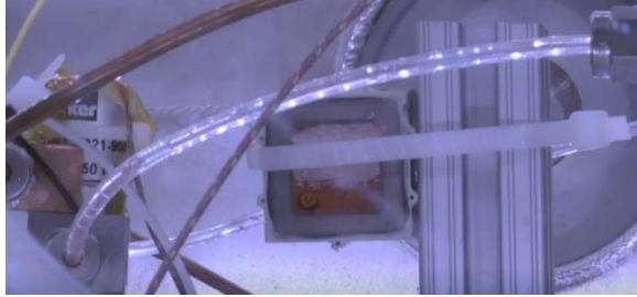
Figure 4. Vapor transfer testing using clear polymer tubing for visualization.
