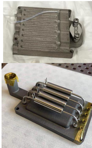
Figure 2. Top: Specter AM Brazed CPRS Design. Bottom: AM Fitting-joint CPRS Design.
