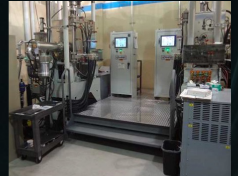
Dual 100-ton Hot Press installed at Teledyne Energy Systems, Inc.
