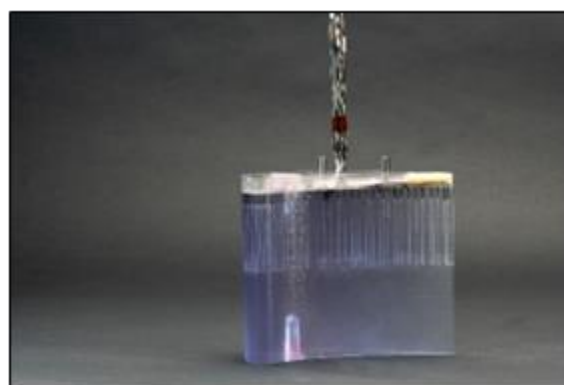
Figure 21: Static Pressure Instrumentation on Baseline Nozzle
