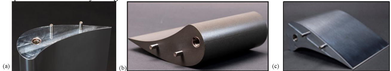
Figure 27: Uninstrumented Test Articles for (a) Baseline (b) Medium and (c) Low Solidity
