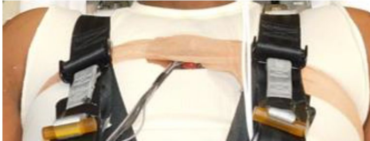
Figure: The chest accelerometer was affixed to subjects with double-sided carpet tape through a hole in their shirt. The accelerometer was wrapped in athletic tape around the torso to provide more stability.
