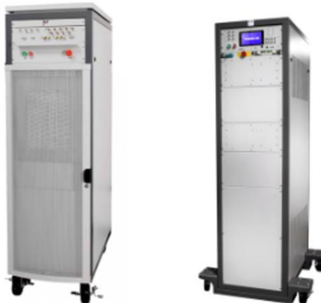
Figure 7: D&V Electronics DC Emulator (Left) and Electric Motor Emulator (Right)
