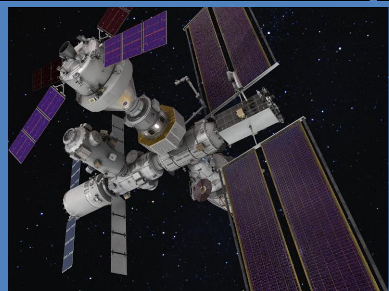
Gateway - Full Configuration in Orbit
