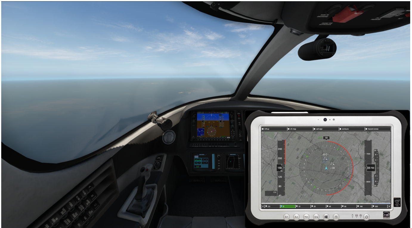
Fig. 4: DANTi prototype integrated with a realistic 3D scenery simulator in NASA's Design Integrity Lab
