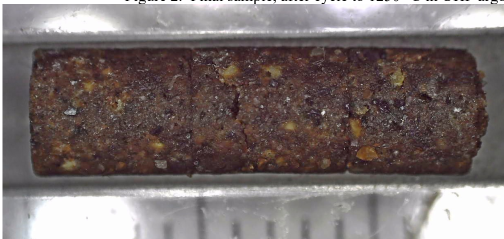
Figure 3. Three final pellets (a “sintered” rod) from 3 rd run—i.e., after the cycle to 1250 °C in UHP argon.
