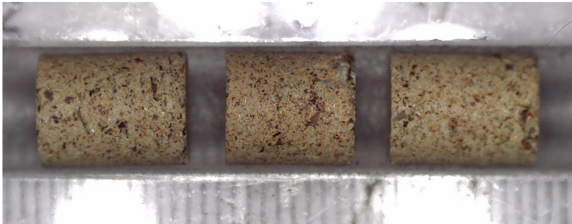
Figure 4. Three final NUW-LHT-5M pellets after a cycle to 1150 °C in UHP argon.
