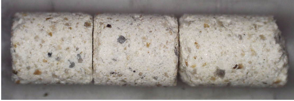
Figure 5. Three final 5M glass pellets after the cycle to 1150 °C in UHP argon.
