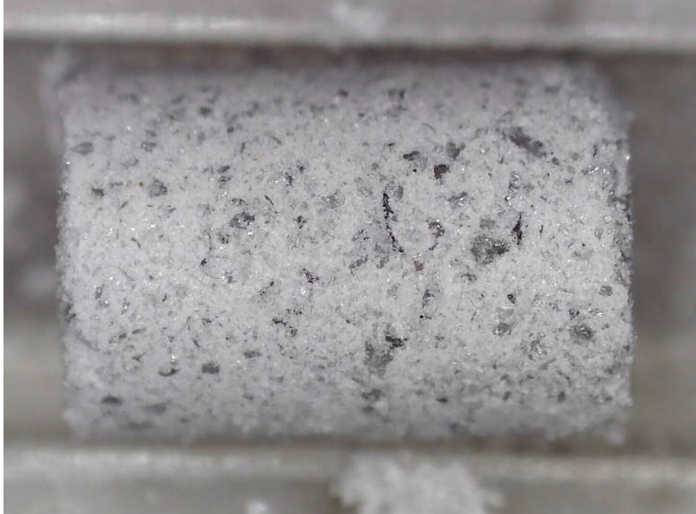
Figure 3. Initial 5M Glass (Washington Mills) pellet pressed at ~33,000 psi.
