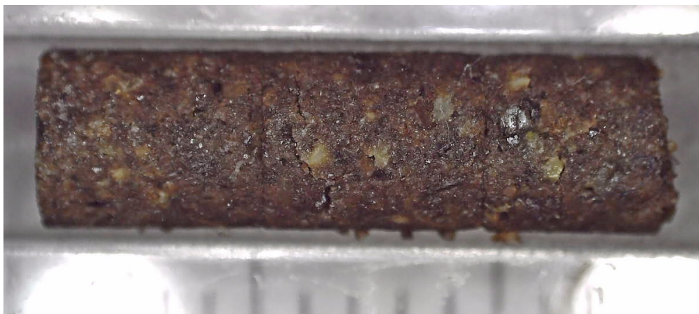
Figure 2. Final sample, after cycle to 1250 °C in UHP argon.
