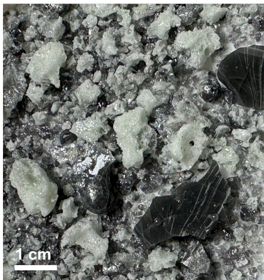
Figure A1. Macro-structure of quenched glass prior to crushing/milling.
